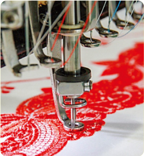
Boring Needle This specifically designed needle creates intricate embroidery by piercing the fabric, cutting it into various shapes, and leaving holes in the item.
